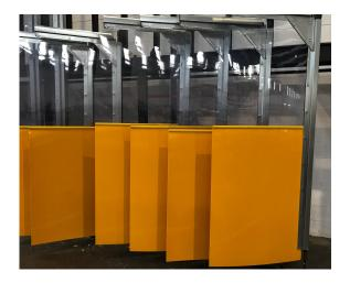
Installation of perfectly flat PVC panels on WINDOR doors frames, is assured by a pre-heating process and vertically mounted on a specific structure. This vouches for many years of reliable door operation with plane plastic panels.
