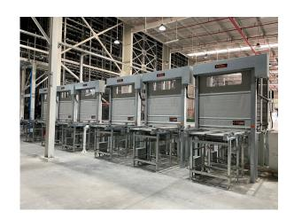
The PAL 150 SPR is specifically designed for integration into automated production systems, with specific safety features and protection of personnel from mechanical hazards (not breakable through).
